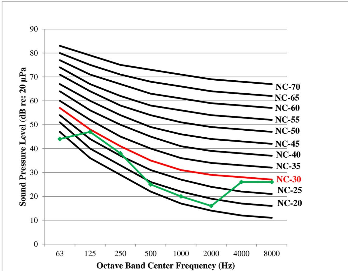
Figure 70: NC plot of background noise level from heat pump duct work for a typical classroom
