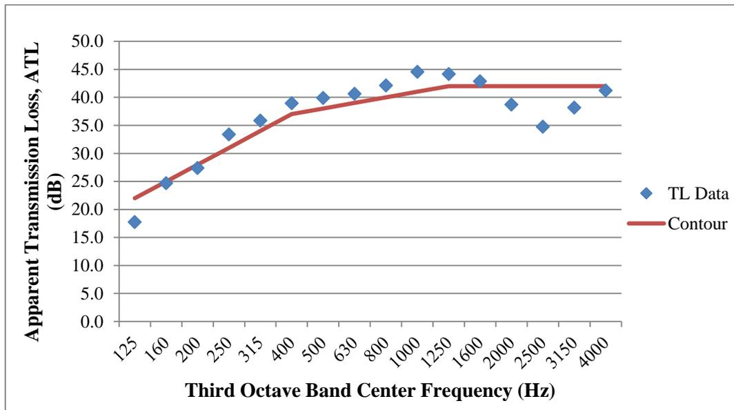
Figure 63: ATL measurement results for the partition between classrooms 247 and 248, with an ASTC of 38
