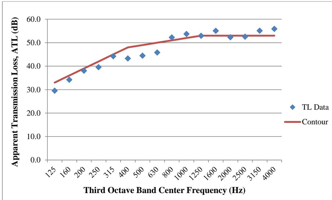
Figure 61: ATL measurement results for the partition between classrooms 121 and 122, with an ASTC of 49
