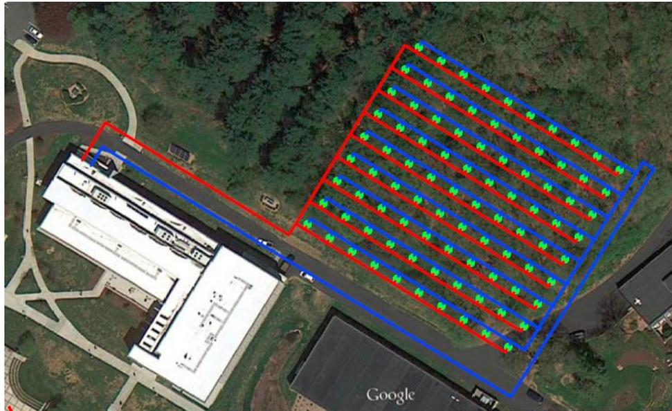
Figure 20: Site layout of the vertical geothermal well field
