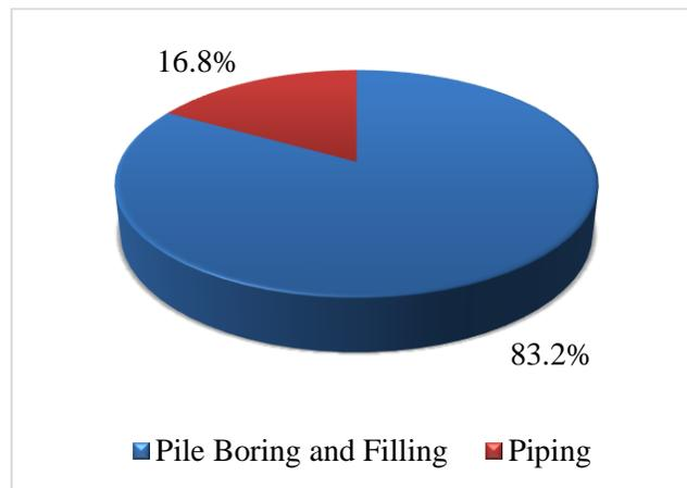
Figure 73: A pie chart showing the percentage breakdown of costs for a vertical geothermal well that is 300’ deep
