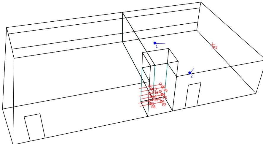
Figure 68: The geometrical model of the two classroom spaces with sources and receivers shown
