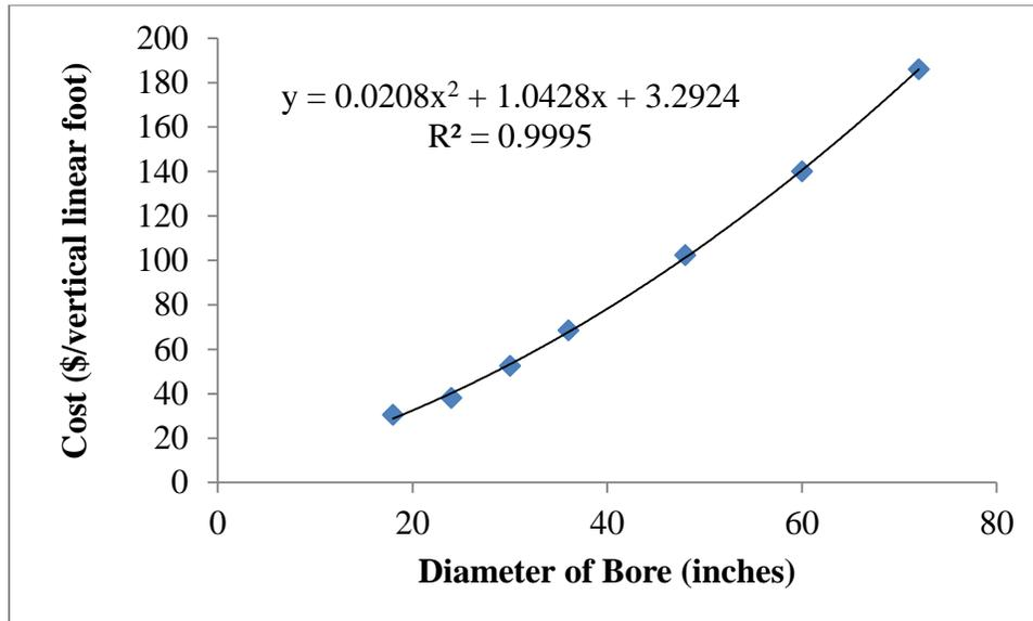
Figure 72: A graph showing RS Means data for pile boring costs as bore diameter changes
