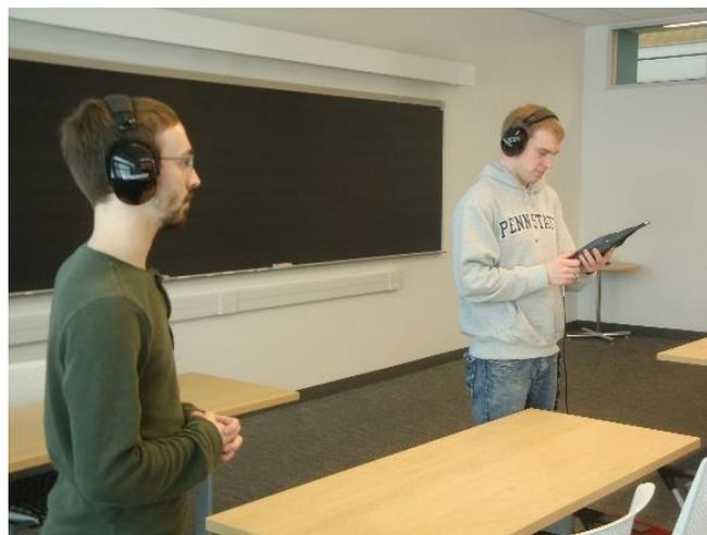
Figure 59: Sound pressure level (SPL) measurements in the ‘source’ room for transmission loss measurements using a B&K 2250 sound level analyzer. (AE 309 students: Aaron King and Cory Clippinger)
