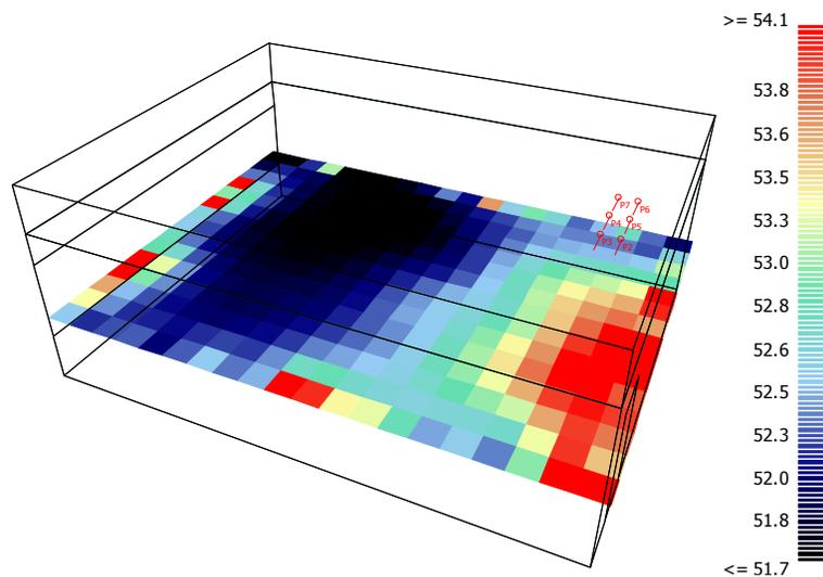
Figure 67: A grid response showing the A-weighted sound pressure levels when heat pump is running in the plenum space above the classroom
