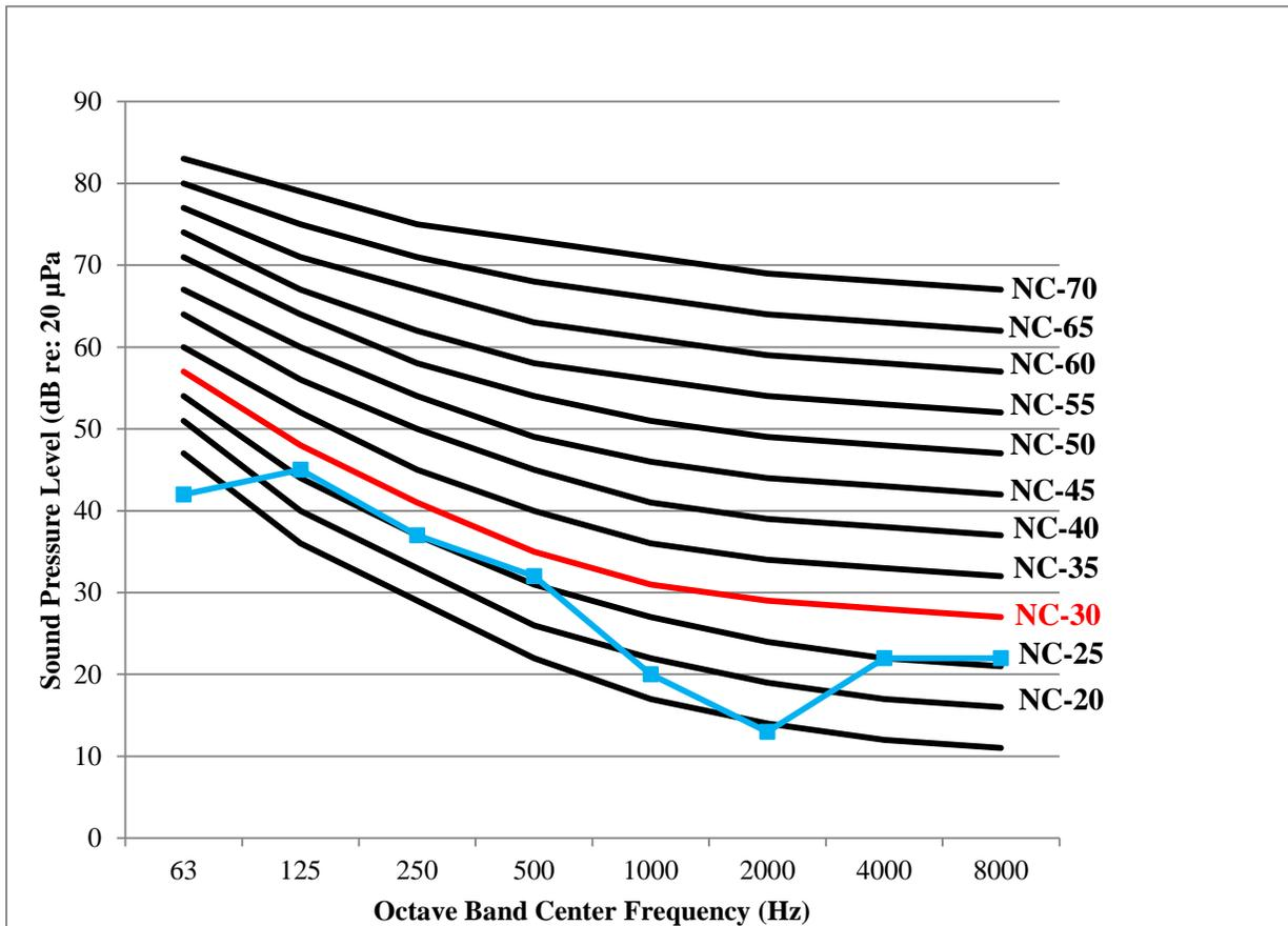
Figure 71: NC plot of background noise level from heat pump duct work for a typical office
