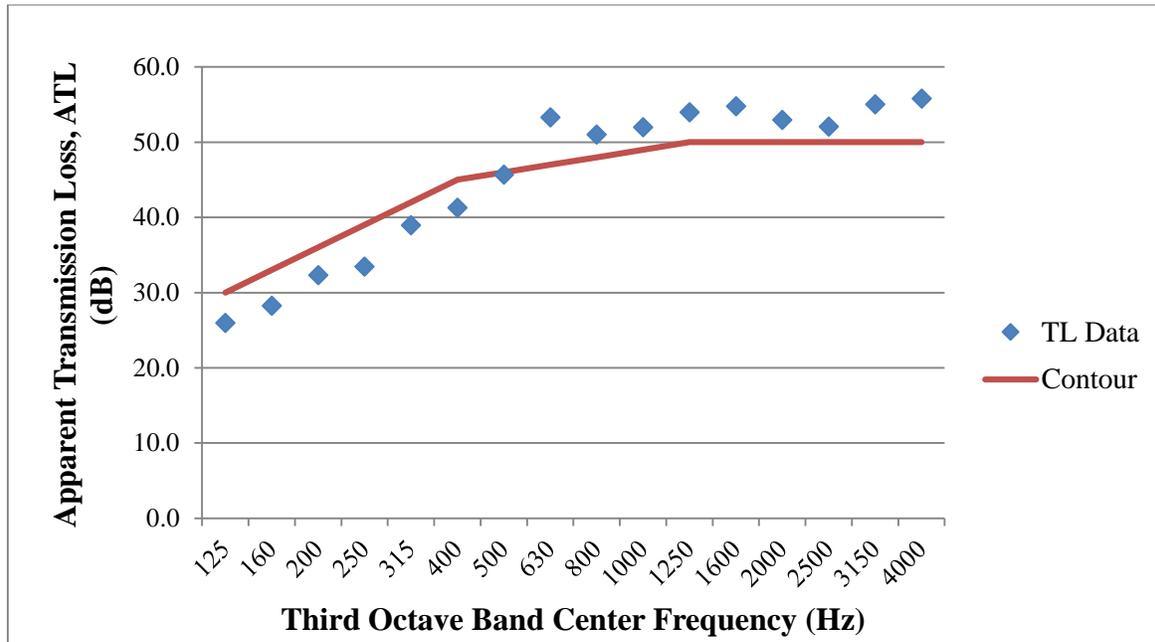
Figure 60: ATL measurement results for the partition between classrooms 120 and 121, with an ASTC of 46
