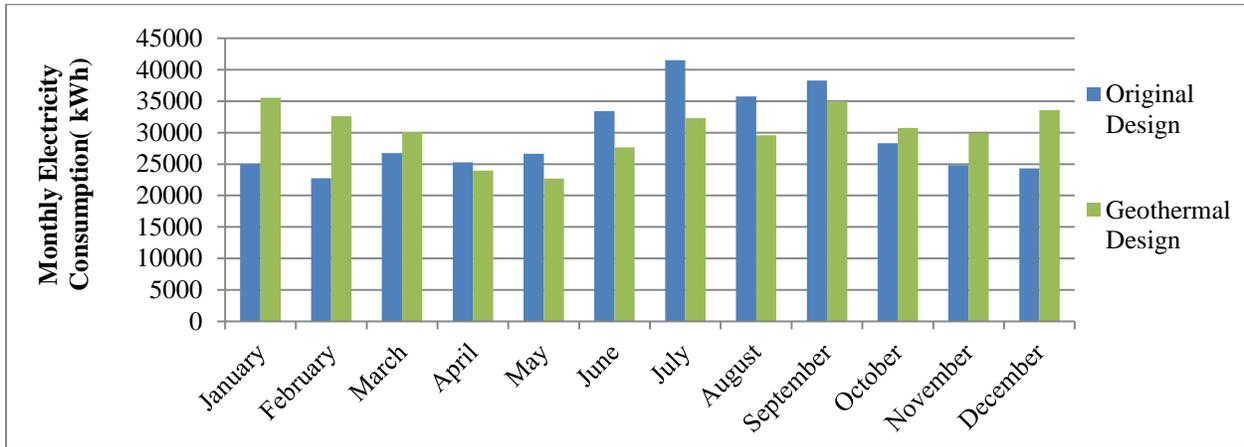
Figure 38: Monthly electricity consumption of the Gaige Building with the original and geothermal redesign
