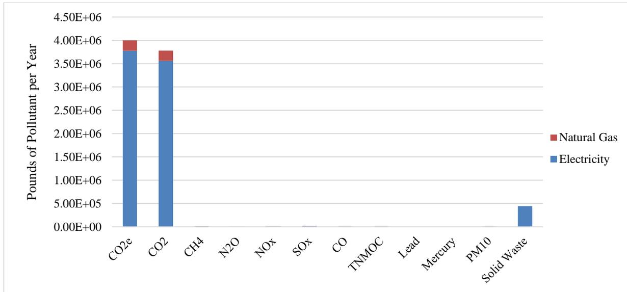
Figure 13: A graph showing the annual emission of each pollutant the Gaige Building by energy source
