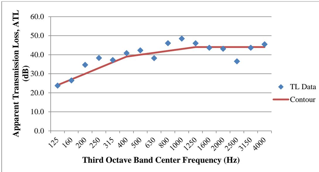
Figure 62: ATL measurement results for the partition between classrooms 246 and 247, with an ASTC of 40
