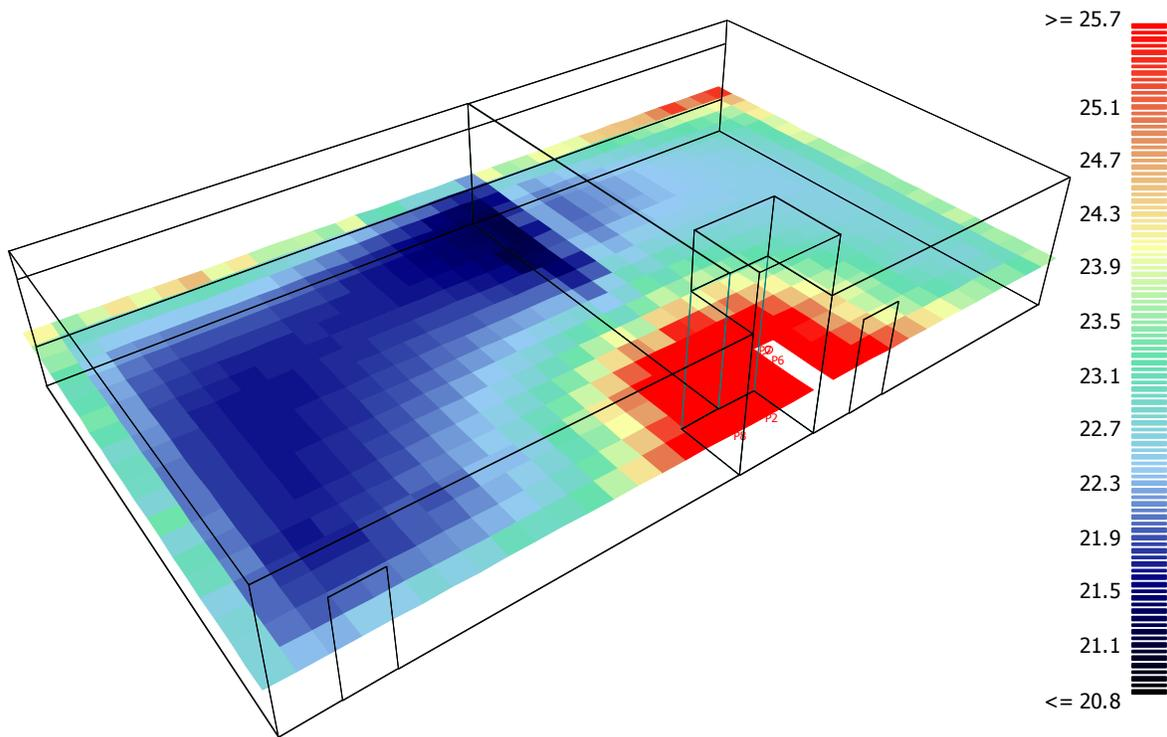
Figure 69: A grid response showing the resulting A-weighted sound pressure levels in both classrooms if two heat pumps were operating within the small mechanical room
