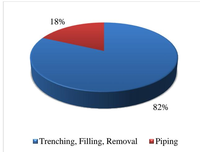
Figure 74: A pie chart showing the breakdowns between trenching and piping costs for a 800' horizontal loop
