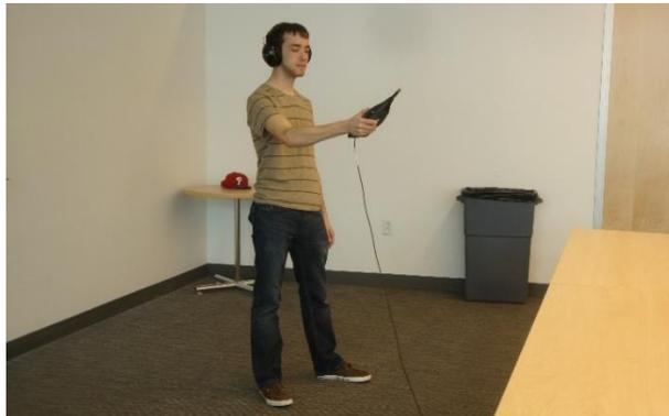
Figure 53: Reverberation time measurement using a B&K 2250 sound level analyzer (thesis author: Matthew Neal)
