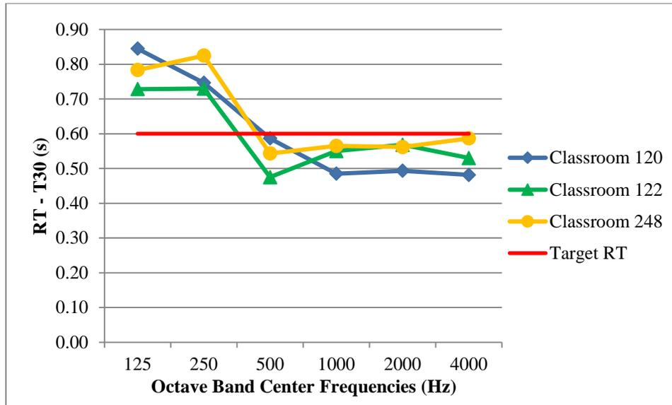
Figure 54: RT measurements of classrooms in the Gaige Building that are less than 10,000 cubic feet
