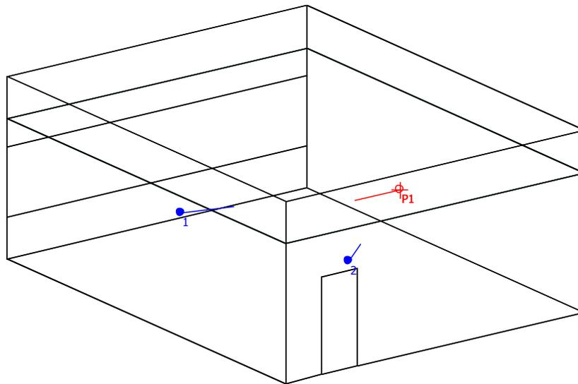
Figure 66: Source location of instructor shown in red, and receiver locations shown in blue, typical classroom
