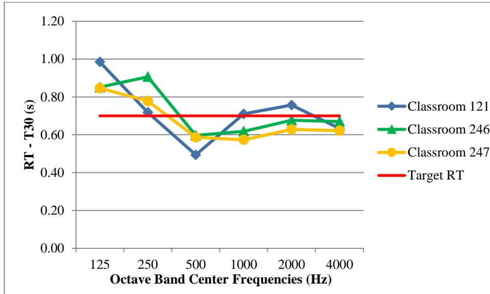
Figure 55: RT measurements of classrooms in the Gaige Building that are greater than 10,000 cubic feet
