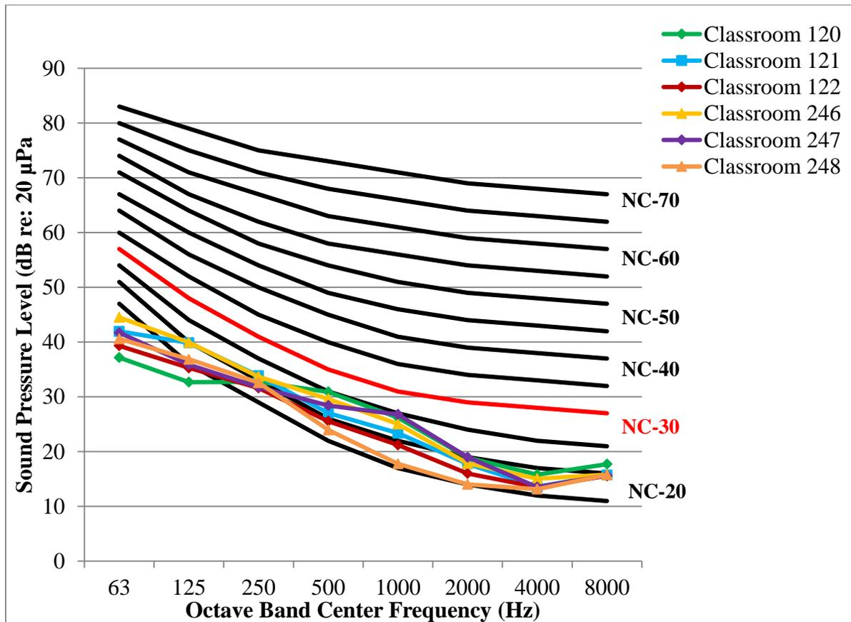
Figure 56: Background noise levels in the six classroom spaces. The target NC-35 is shown in red
