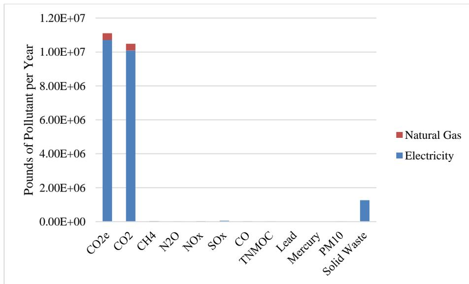
Figure 52: Estimated annual emissions from the geothermal redesign of the Penn State Berks campus
