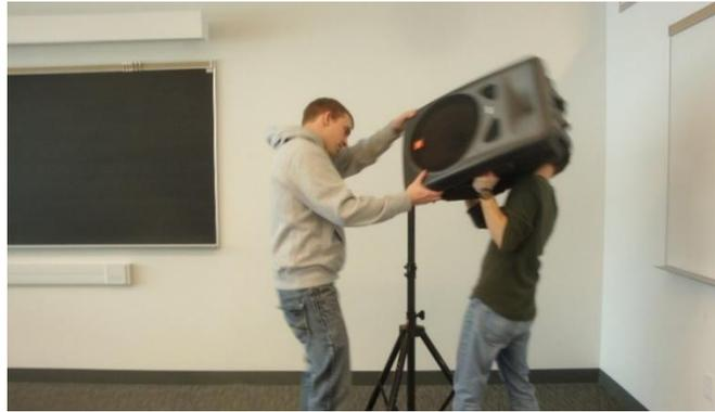
Figure 58: Setting up JBL speakers in the ‘source’ room for the transmission loss measurements (AE 309 Students: Aaron King and Cory Clippinger)
