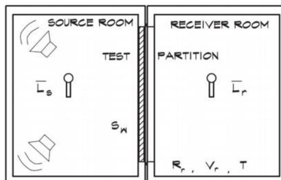
Figure 57: Typical measurement setup to take transmission loss measurement of a partition between rooms (Graphic from *Architectural Acoustics* by Marshall Long, with modification Michelle Vigeant)
